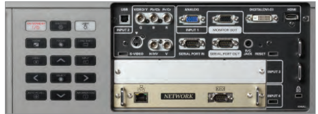
Complete local control, professional inputs, network module & expansion bay.
